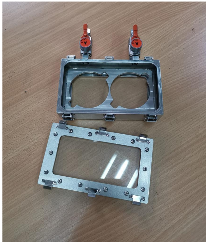
Fig. 2: Component parts of the miniature incubation chamber (MIC)
