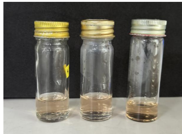
Fig 5: The nutrient broths inoculated with Cellcure® embryo culture medium were clear, with no visible turbidity. Similar observations were noted for remaining gamete and IUI media.
